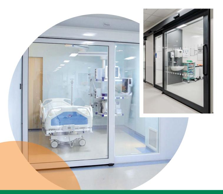
If greater visibility is desired for the hermetic glazed door, a fixed leaf can be added, when it is single slide door, or two fixed leaves for a bi-parting door. Hence, patient visibility is maximised and virological contamination is minimised.
